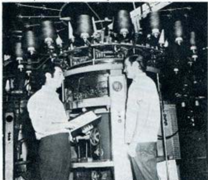
David Adelman, left, talks over production matters with knitting foreman, Wildman. Jacquard machine shown here is used for production of tubular knit fabric for golf sweaters.
