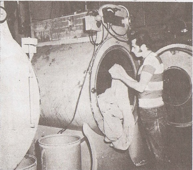
All knitted fabrics produced here are washed to take out initial shrinkage, eliminate oil content and improve the hand of the end product.
